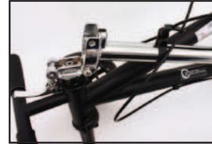
Push the unfolded steering column clamp inward, to the left, to release the steering column. Once the steering column is released, it will be able to fold forward in a laid-down position.
