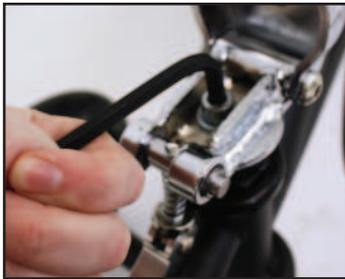
Make sure to stop wheel/overall scooter movement while tightening screw in order to ensure reset alignment does not change.
