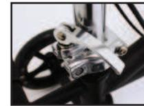
Use a clockwise motion until clamp feels tight, then push clamp downward.
